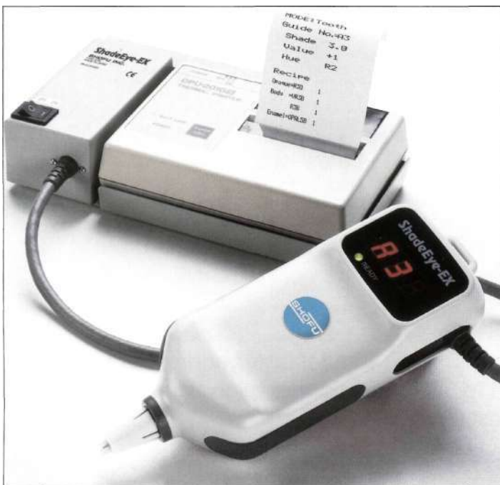
Fig 5-71 The Shofu ShadeEye-EX Chroma Meter (Shofu, Menlo Park, CA) uses a single point source spectrophotometer as the basis of shade analysis.
