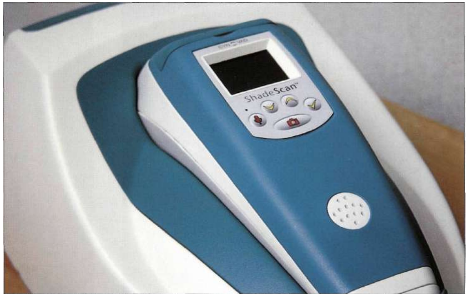
Fig 5-72 The ShadeScan System (Cynovad, formerly Cortex Machina, Montreal, Canada) uses computer-aided digital camera vision technology to analyze dental images and infer color and translucency.
