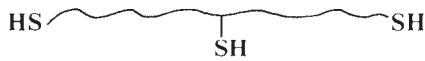
Fig. 19.2 Simplified structural formula of the polysulphide prepolymer showing terminal and pendant –SH groups.
