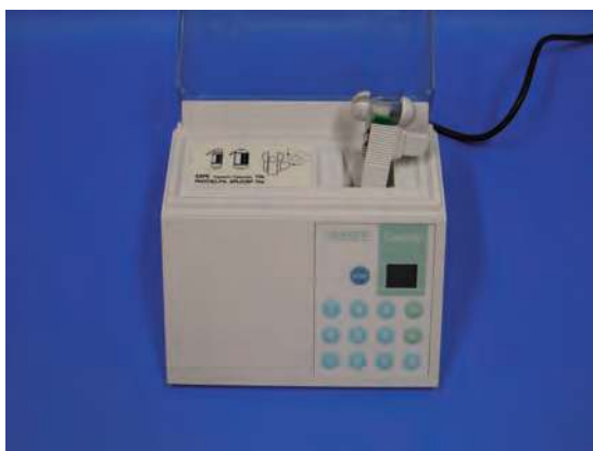
Fig. 24.3 A mixing device that can be used for mixing a number of materials including dental cements. Mixing is achieved by rapid shaking of a capsule. Typically glass ionomer cements as shown in Fig. 24.2 are mixed on this sort of instrument and mixing times may vary between 5 and 15 seconds.
