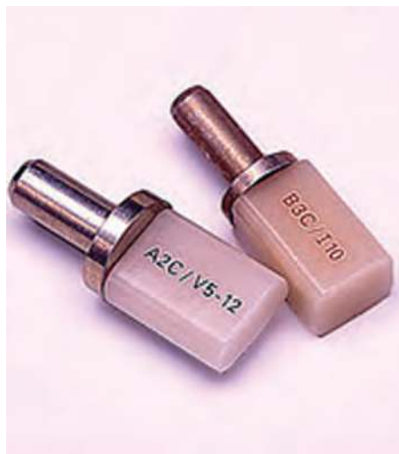
Fig. 11.5 Materials for CAD–CAM restorations. This shows blanks of materials which are used for milling the shapes required in the CAD–CAM milling machine shown in figure 11.3. The metal part of these blanks is held in the grips of the milling machine and the tooth coloured parts (ceramic or resin based) are milled to the correct shape. Figure reproduced with permission of www.planetcerec.com .
