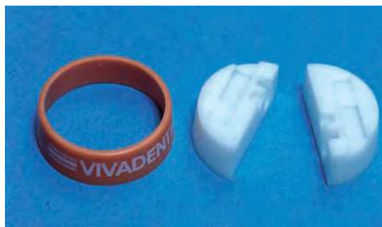
Fig. 22.10 A 3-part mould of this sort can be used by the dentist to make an estimate of depth of cure. The mould is assembled and composite material is packed into the cavity and cured by exposure to a curing lamp. The mould is then disassembled and a probe can be used to estimate the depth at which material remains soft. Regular determinations can be used to confirm that both material and curing equipment are in good order.
