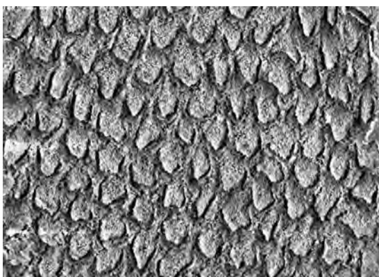
Fig. 23.1 Scanning electron micrograph of the surface of enamel after etching with 37% phosphoric acid followed by rinsing and drying ( \times 2000 magnification).
