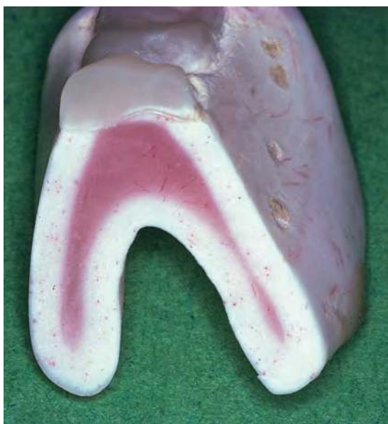
Fig. 13.11 Whitened denture base. This shows a section through a denture base which has been whitened by the patient using an oxygenating cleanser in hot water (>90°C). The original colour of the denture can be seen in the middle of the section and we can see that the whitening effect has progressed inwards from the outside surface. The original pink colouration of the veins which are present in this material can also be seen.
