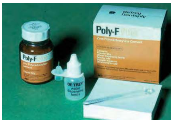
Fig. 30.1 A polycarboxylate cement. The cement contains two main reactive ingredients, zinc oxide and polyacrylic acid and both are in the powder; the bottle is filled with water by the dentist. Powder and water are dispensed onto the mixing pad and mixed with a spatula. In other products the powder contains only the zinc oxide and the liquid is an aqueous solution of polyacid.
