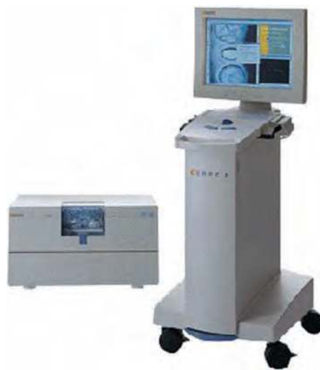
Fig. 11.3 CAD–CAM generated dental appliances. This shows a CAD–CAM equipment set up for manufacturing dental appliances and restorations at the chairside using computer generated images and computer controlled milling equipment. On the right of the figure is the control unit and the computer which is used for viewing the scanned images and on the left is the milling instrument in which the shapes are cut from a variety of materials. Figure reproduced with permission of www.planetcerec.com .
