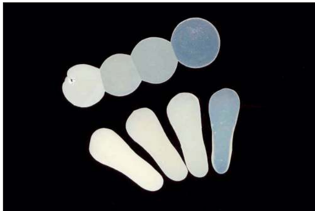
Fig 10-4 Resin composite increments of the same thickness presenting four opacities: Dentin, Body, Enamel, and Translucent (Filtek Supreme Ultra, 3M ESPE).
