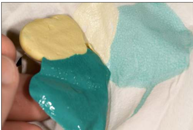
Fig 18-36 The staining of a latex glove indicates inhibition of polymerization of polyvinyl siloxane impression material.
