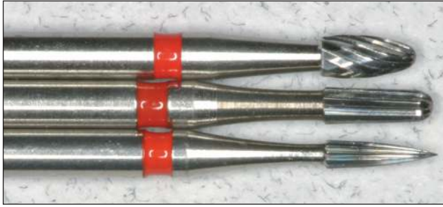
Fig 12-75 Finishing burs for a friction-grip handpiece: (top to bottom) no. 7404 (bud or egg shaped), no. 7803 (bullet shaped), no. 7901 (needle shaped).
