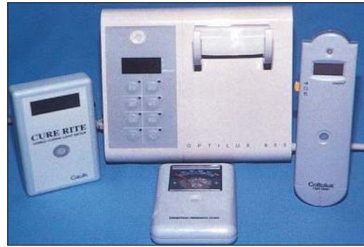
Fig 11-46 Commercial radiometers available to monitor adequacy of irradiance of visible light-curing units. (Courtesy of USAF Dental Evaluation and Consultation Service.)
