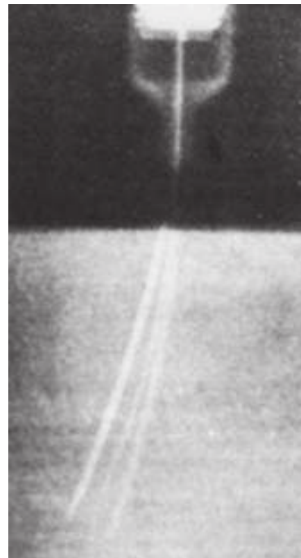
• Fig. 6.4 Radiograph demonstrating various degrees of needle deflection with different gauges (from left to right, 30 gauge, 27 gauge, and 25 gauge). (From Robison SF, Mayhew RB, Cowan RD, et al. Comparative study of deflection characteristics and fragility of 25-, 27-, and 30-gauge short dental needles. J Am Dent Assoc. 1984;109:920-924.)
