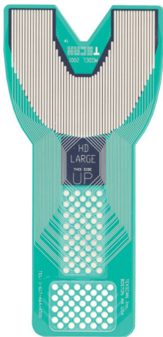
Figure A1.4. T-Scan III Sensor Schematic. Reprinted with permission from Tekscan, Inc. www.tekscan.com/dental .
